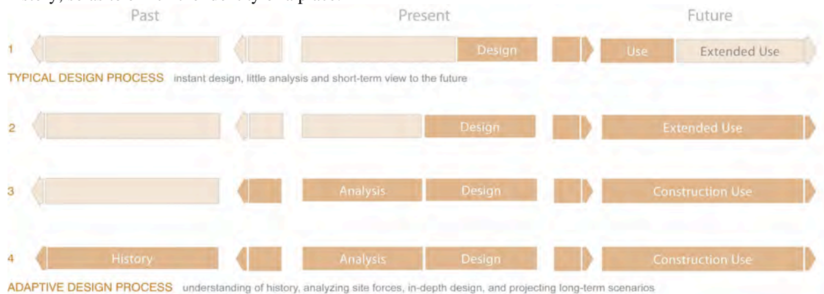
Figure 1. A schematic diagram compares implementation of a typical design process with the implementation of the Adaptive Design Process
