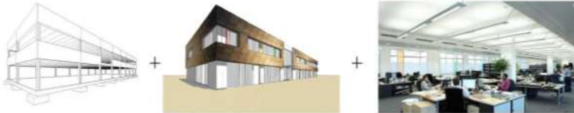
Figure 2: The skeleton, the skin and the fit-out
