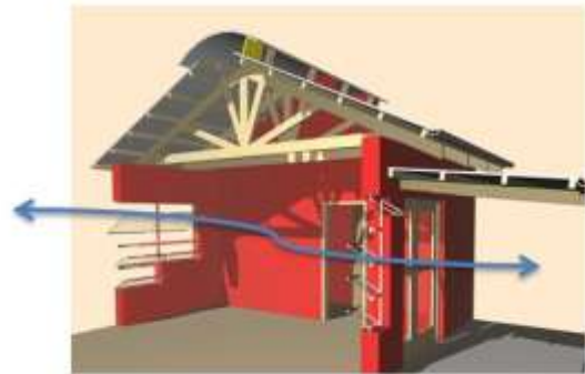
Figure 5. Ventilation criteria in TB wards. (Source CSIR)
