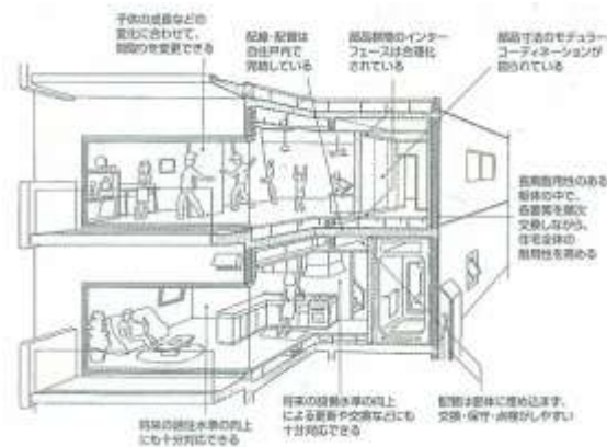
Figure 2 Century Housing System (CHS) Concept drawing*2 Actually, CHS is proposal, but some parts are involved in the actual projects. Infill is installed under modular coordination, dimensions between wall to wall are 300n.
