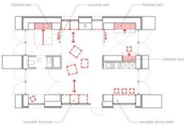
Figure 5: +hytte: third delivery. Boxes are reduced to the minimum into long functional cells in order to rationalize the transport process.
